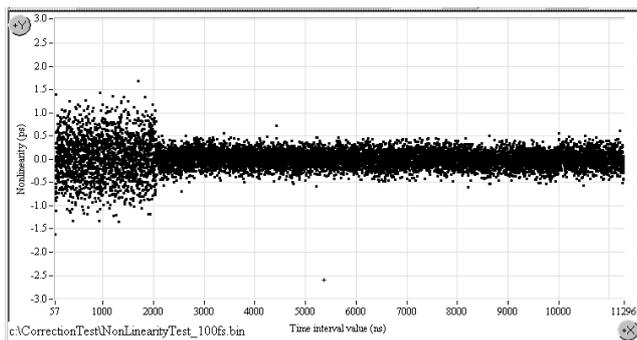
**Fig.6.** Evaluated linearity function after correction
