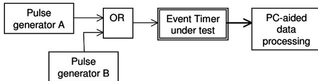
Fig.1. Test circuits for linearity evaluation
