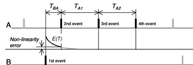
Fig.2. Time diagram of measured events arriving
