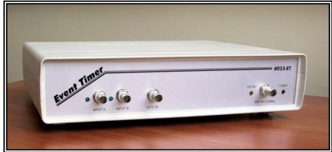
The A033-ET offers two inputs (A and B) to measure events on these inputs alternately with 50 ns dead time. Result of every single measurement (epoch time-tag) is represented in digital form with 1 ps LSB resolution. Time-tags appear at the timer's output in order of event measurement. Special mark accompanies each time-tag, indicating the input that provides measured event. There are two basic operation modes for such measurement:
