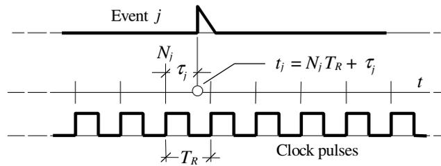
Fig. 1. Combined timing principle.
