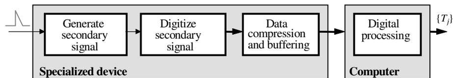
Fig. 4. Typical structure for a measurement system based on the EET method.
