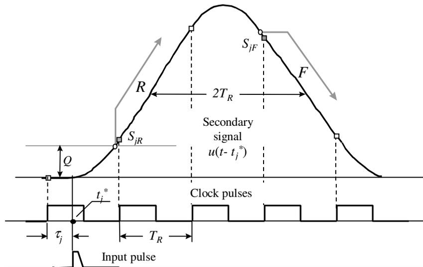
Fig. 2. Example of a quasioptimal secondary signal waveform.
