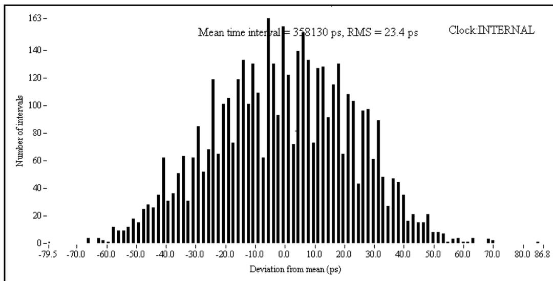
**Fig. 8. Histogram for output signal period measurement for a highly stable crystal oscillator.**
