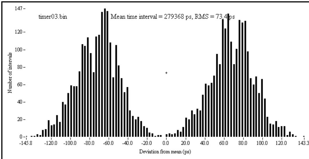
**Fig. 7. Histogram for output signal period measurement for a typical crystal oscillator.**
