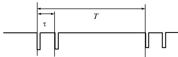
**Fig. 3.** The waveform diagram for the timer input signal.
