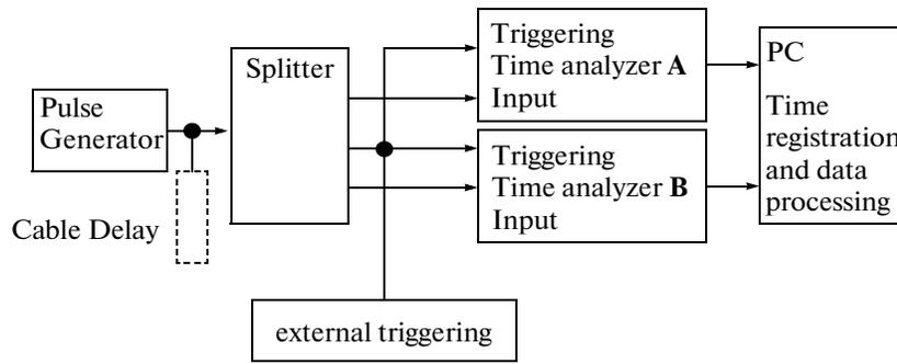
Fig. 1. A block diagram of the measuring system for the implementation of the correlation method. The dashed line shows the delayed pulse generator at the open segment of the coaxial cable.
