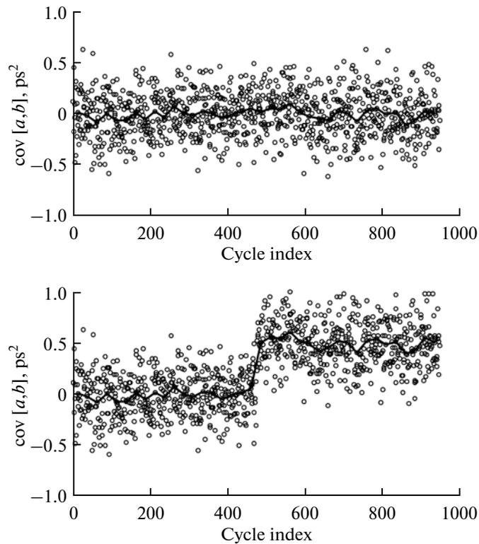
**Fig. 5.** The covariance of the meter errors in the computer simulation. The points connected by the solid line show the averaged results of 25 cycles (16 000 measurements in a cycle). The top graph shows the mean value of  $\overline{\text{cov}[a,b]} = 0.003 \text{ ps}^2$ ,  $\sigma_{\text{cov}[a,b]} = 0.22 \text{ ps}^2$ . In the bottom graph, the correlation of errors of  $0.5 \text{ ps}^2$  is introduced after 500 cycles.
