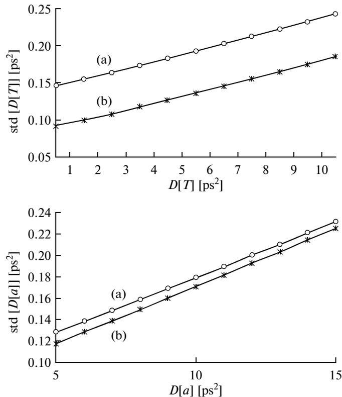
**Fig. 2.** The results of computer simulations on the dependence of the evaluations of the standard deviations of  $D[T]$  (top panel) and  $D[a]$  (lower panel) on the values of the variances. Lines (a) refer to the three-cornered hat method. Lines (b) refer to the correlation method.
