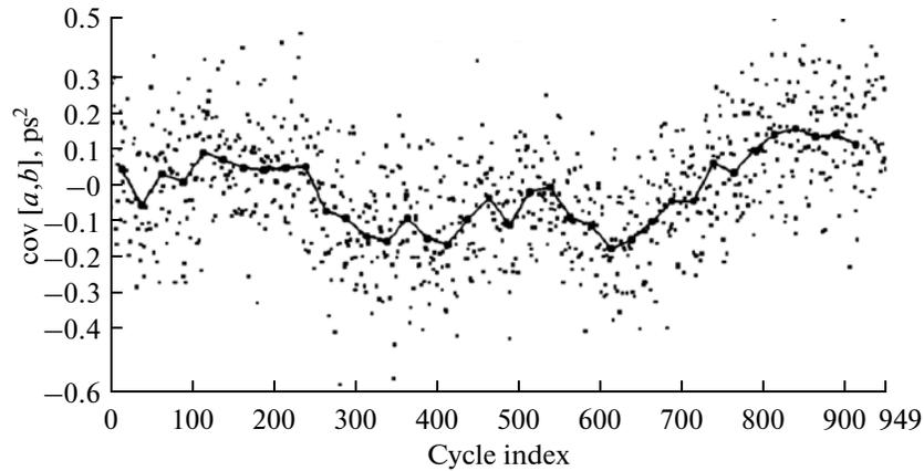
**Fig. 4.** Covariance of errors of the A033-ET timers. The points connected by the solid line show the averaged results of 25 cycles (16000 measurements in a cycle). The mean value across the whole sample is  $\overline{\text{cov}[a,b]} = -0.0109 \text{ ps}^2$ ,  $\sigma_{\text{cov}[a,b]} = 0.16 \text{ ps}^2$ .
