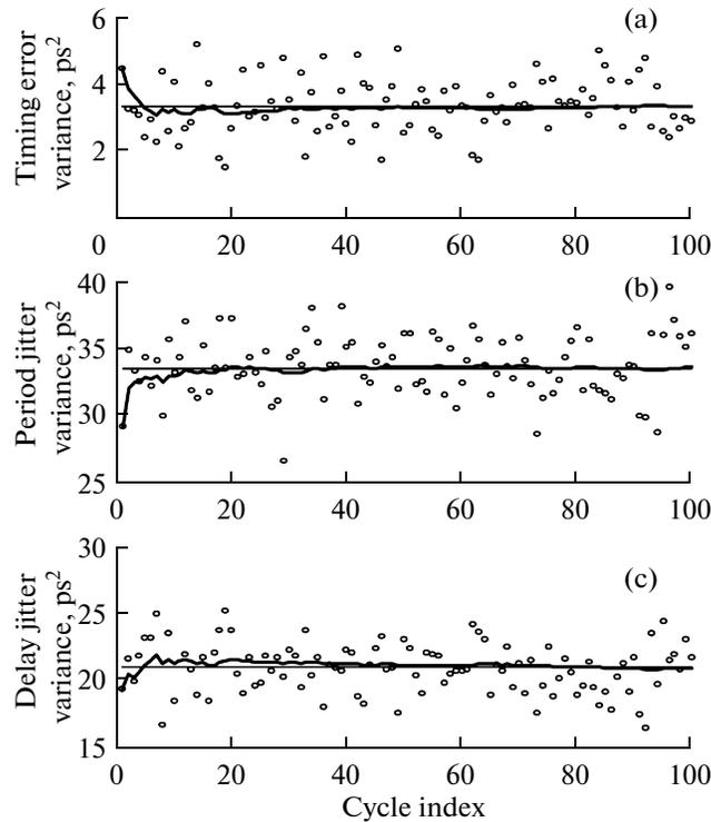
**Fig. 5.** Dependences of the current averaged estimates for the timing error variance (*upper panel*), the event repetition period jitter variance (*middle panel*), and the delay jitter variance (*lower panel*) on the number of measurement cycles. The circles show the variance estimates in each cycle. The dashed horizontal lines show the set values of the variances ( $3.4 \text{ ps}^2$ ,  $33.9 \text{ ps}^2$ , and  $21.4 \text{ ps}^2$ ). It is a quasi-periodic event flow.
