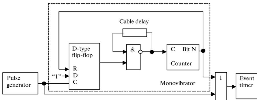
**Fig. 6.** Timing error experiment procedure.
