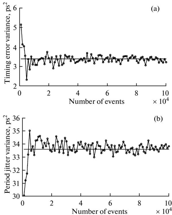
**Fig. 3.** Example of dependences of timing error variance estimates (*upper panel*) and period jitter variance estimates (*lower panel*) on the number of events (Palm flow). The dashed horizontal lines show the given values of the variances ( $3.4 \text{ ps}^2$  and  $33.9 \text{ ps}^2$ ).
