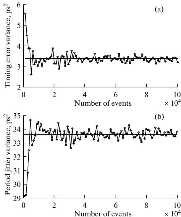
**Fig. 2.** Example of dependences of timing error variance estimates (*upper panel*) and period jitter variance estimates (*lower panel*) on the number of events (quasi-periodic event flow). The dashed horizontal lines show the given values of the variances (3.4  $\text{ps}^2$  and 33.9  $\text{ps}^2$ ).
