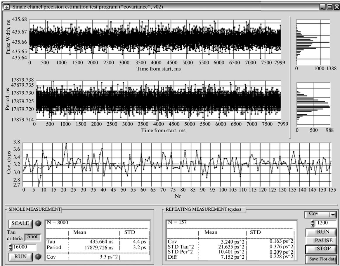
**Fig. 8.** Results of the study of the period jitter for the EXO-3 crystal oscillator with a frequency of 14.383 MHz and a denominator of 256.
