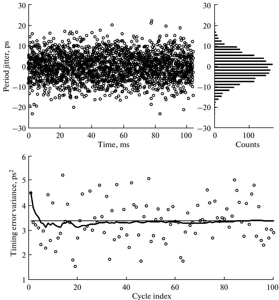
**Fig. 4.** Period jitter for events of the quasi-periodic flow in one cycle (*top left*), a distribution histogram for the period jitter (*top right*), and the dependence of the current averaged timing error variance estimate on the number of measurement cycles (*lower panel*). The circles in the lower panel show the variance estimates in each cycle. The dashed horizontal line shows the set values of the timing error variance ( $3.4 \text{ ps}^2$ ).
