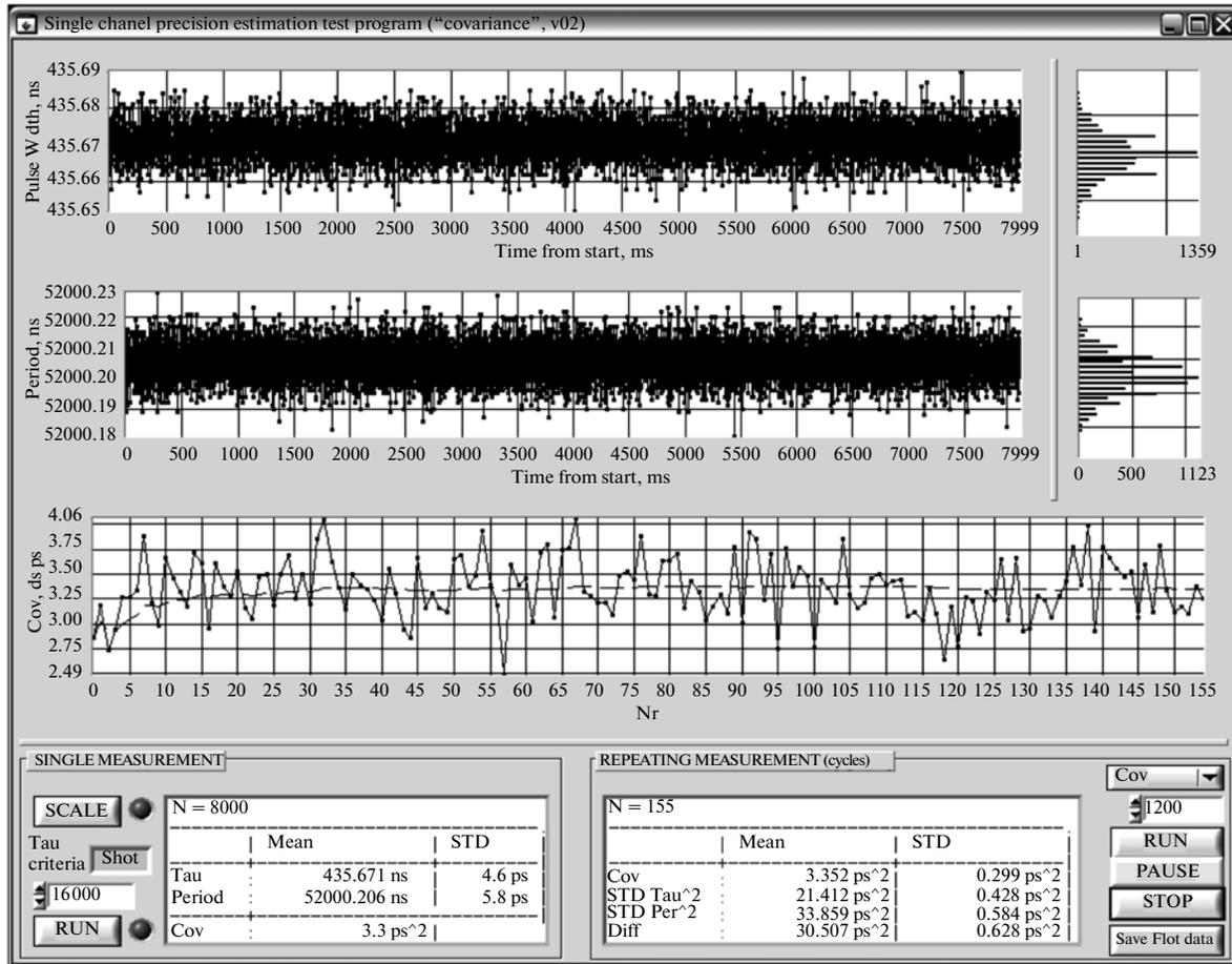
Fig. 7. Results of the timing error experiment with an AFG3252 generator.
