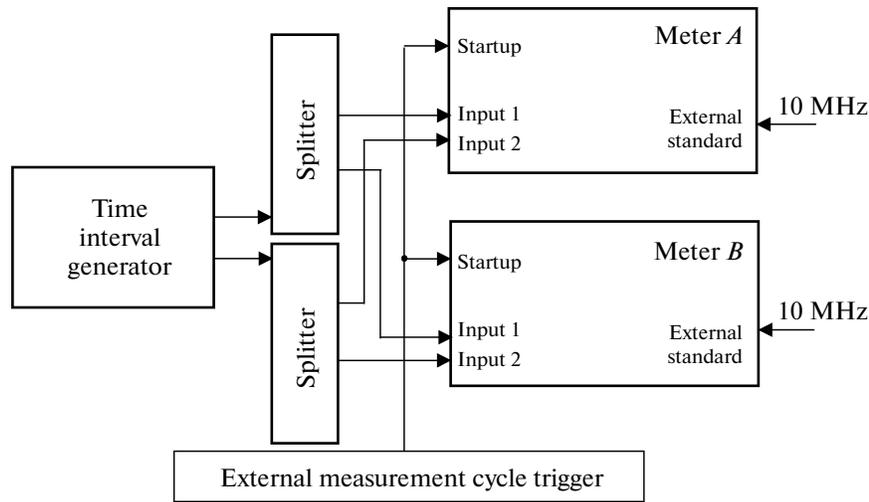
Fig. 3. Block diagram for parallel measurements by two meters.
