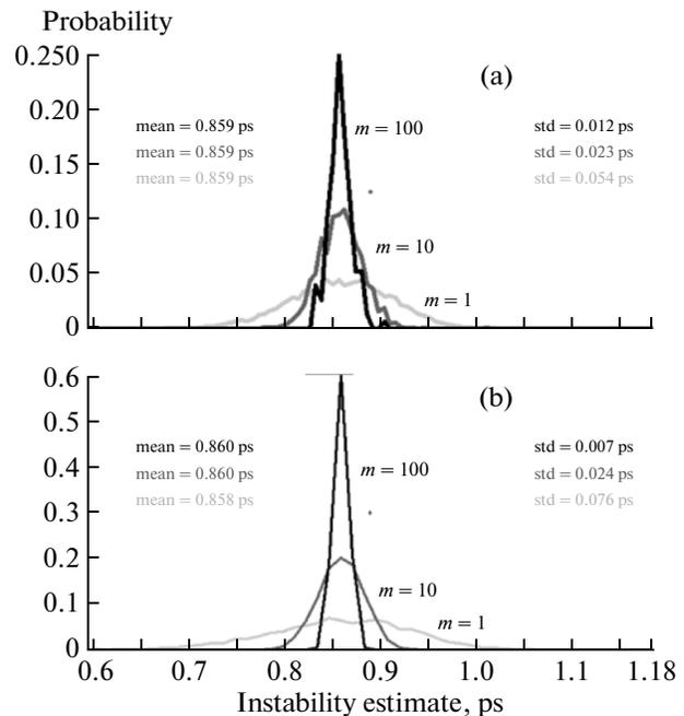
**Fig. 5.** Instability estimate of the time intervals generated by the generator based on the quartz VCO from the FORDAHL Co. (the TI value is 40.96  $\mu\text{s}$ , the repetition period is 81.92  $\mu\text{s}$ , and  $m$  is the number of averaged cycles): (a) actual measurements and (b) computing experiment.
