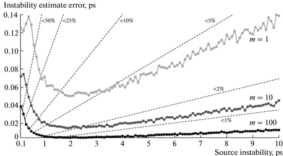
**Fig. 6.** Simulation results of the dependence of the error of the instability estimate on its value for  $m = 1, 10,$  and  $100$ . The bounds of the relative estimate error are shown from 1 to 50%.
