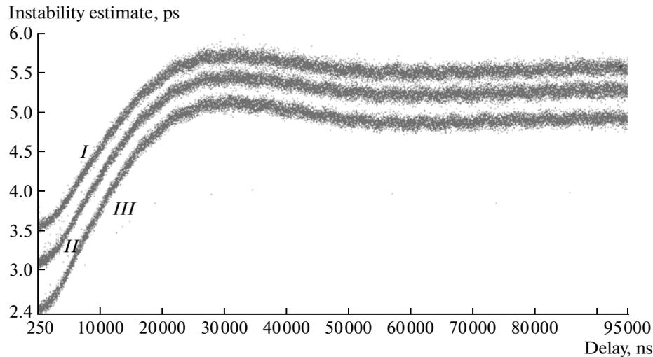
**Fig. 2.** Instability estimate of the delay between channels of the AFG3252 generator in a delay range of 250 ns–95  $\mu$ s (the step is 5 ns,  $n = 3000$ ): (*I*) from the dispersion of measurement results obtained by one meter; (*II*) from the dispersion of the half-sum of the simultaneous measurement results by two meters, and (*III*) from the covariance of the simultaneous measurement results by two meters. The TI repetition period is 100  $\mu$ s.
