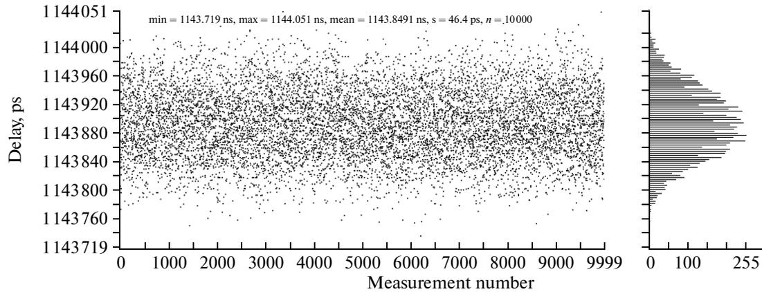
**Fig. 1.** Measured instability of TIs with durations of 1143 ns, generated by the И1-8 time shift source (measured TI train is on the left, and the measured data distribution histogram is on the right).
